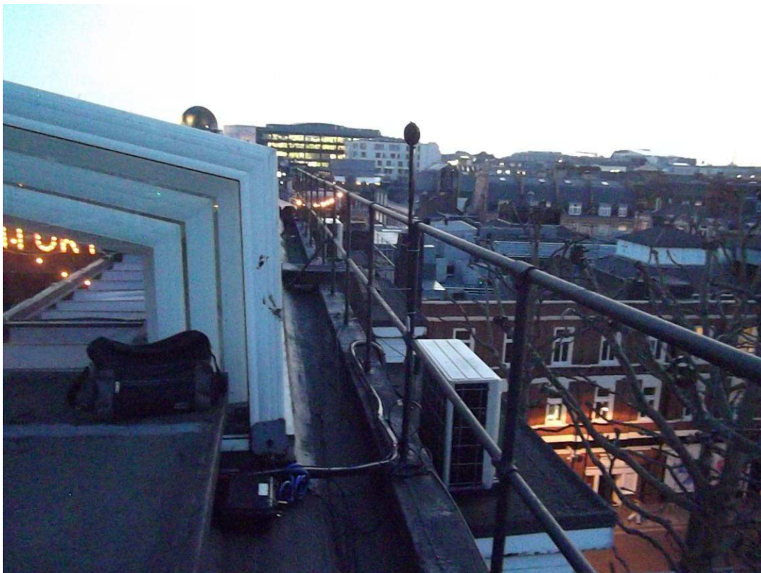
Figure 4: Noise logging position on balustrade at edge of roof canopy.
